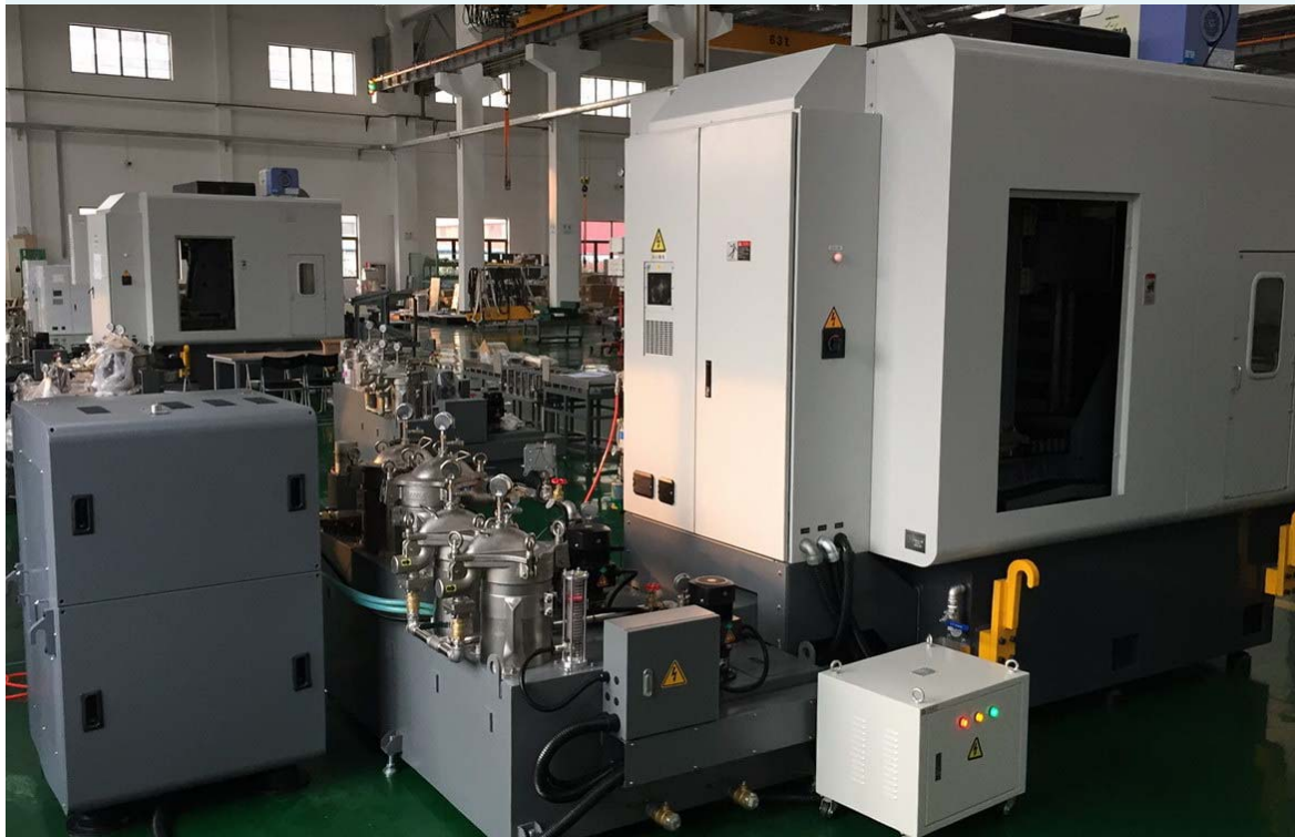
7,000 PSI Pumping Sysem with Multistage Filtration System
